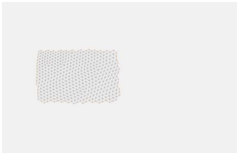
Figure 13. Bathymetry scatterset generated from master grid that is later interpolated to re-meshed portion of the grid.
