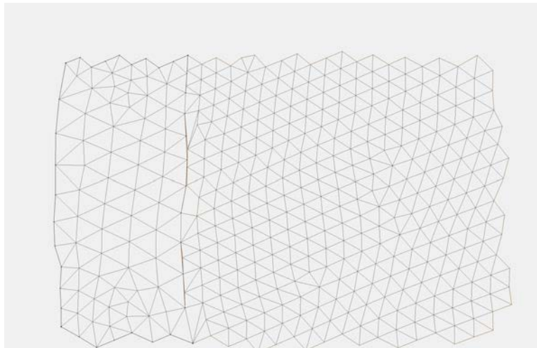
Figure 15. Grid with unsuccessful re-meshed area
