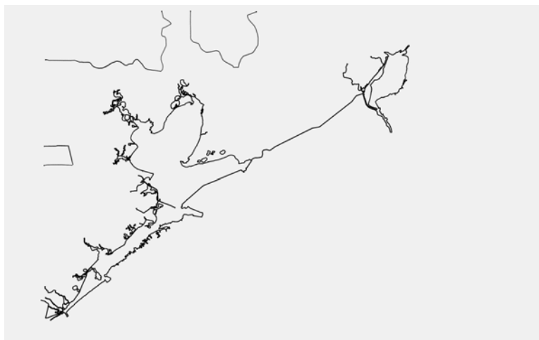
Figure 5. Polygon built from nodestrings delineating Galveston Bay and Sabine Lake.
